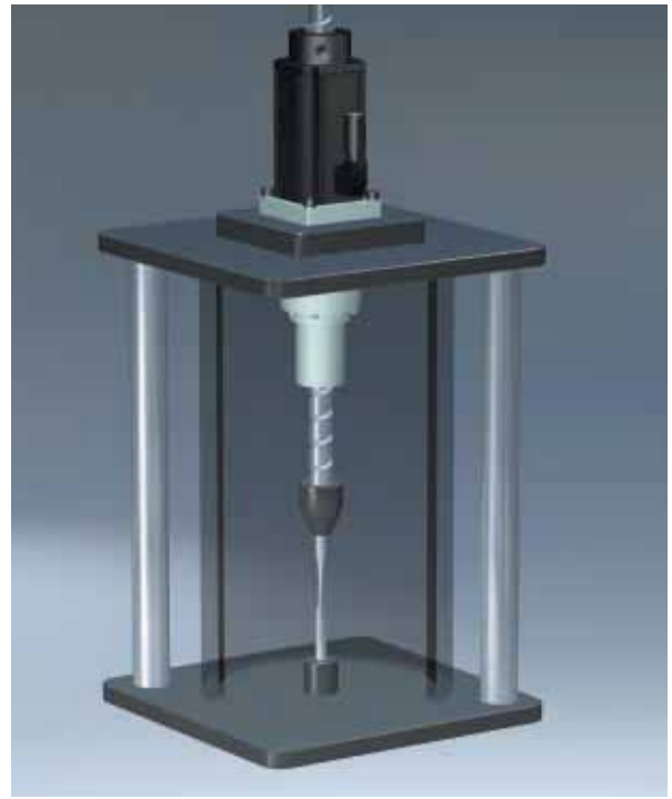
▲ Tensile testing with M HS drive unit
