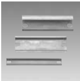
Mounting rails TS-32 and TS-35, steel, yellow-passivated for terminal block attachment.
