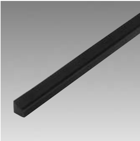
Profiled sealing strip (Part number 980.8.0099.00) Profiled strip made of silicone for sealing gap between front plate and enclosure. Simple to cut to the required length and fit before mounting front plate.
