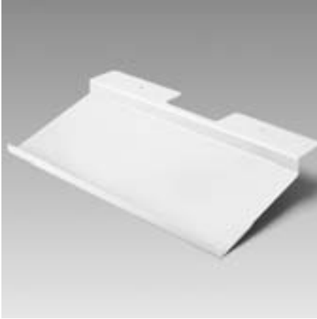
Keyboard shelf (Part number 980.6.1750.00 painted sheet steel) (Part number 980.6.1760.00 VA 1.4301) sheet steel keyboard support for subsequent mounting, RAL 7035, light grey, 10° inclination; mechanical machining is required for mounting. Attachment material is included.
