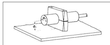
Installation with mounting flange parallel to a steel wall or surface.
