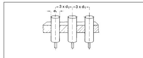
Minimum distance for the non-flush installation of sensors.
