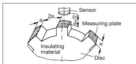
The distance between the measurement plates and the sensor is half of the nominal sensing distance. The maximum switching frequency is achieved when the switch-on/off output signal falls below 50 ms.
