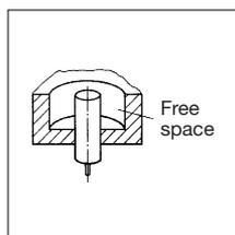
Sensors for non-flush installation must be provided with a free zone, which is three times greater than the diameter of the active surface and 25 mm thick. Catalogue symbol for non-flush installation.
