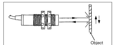
Diffuse reflective sensors have the light source and receiver in the same head. The light emitted by the source is diffusely reflected by the detected object. A part of this reflection returns to the receiver and changes the switching status of the output when a certain intensity is exceeded. Thus the texture and colour of the object's surface has a great effect on the detection (presence/absence) of objects.
