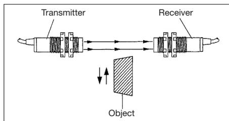
Through-beam sensors have the light source and receiver in separate heads. The light emitted by the source is analysed by the receiver. Interruption of the light path (caused by an object) is evaluated and results in switching of the output.
