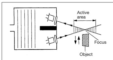
The transmission and reception elements of convergent beam sensors are arranged in a defined angle to each other. The light cone of the source and the receiver are joined in a fixed focal point. This results in the active zone for the detection of objects being defined around this focal point.
