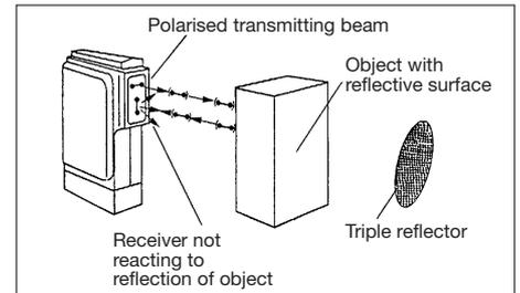
This device is a special type of retro-reflective sensor. Special linear or circular polarised filtering elements (foils) are mounted between the reception/transmission elements and the lens of the sensor.
