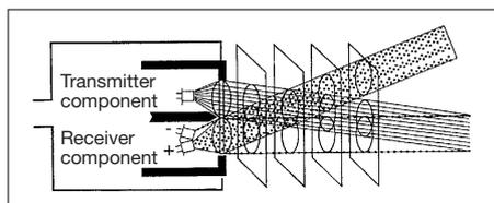
This type of sensor is a special type of diffuse reflective sensor. It is based on two receptive elements (segmented receivers). Using the triangulation principle, reflections of objects beyond the target do not reach the active surface of the receiver modules.
