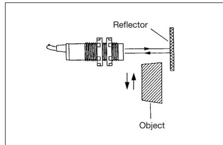
Retroreflective sensors have the light source and the receiver in the same head. The light beam emitted by the source is reflected back to the receiver by a reflector (e.g. triple reflector or reflective foil). Any break in the light path is evaluated by the receiver and in turn results in a change of the output mode.
