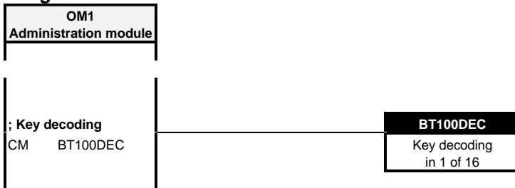
Fig. 4-29 Program Structure, Key Decoding
