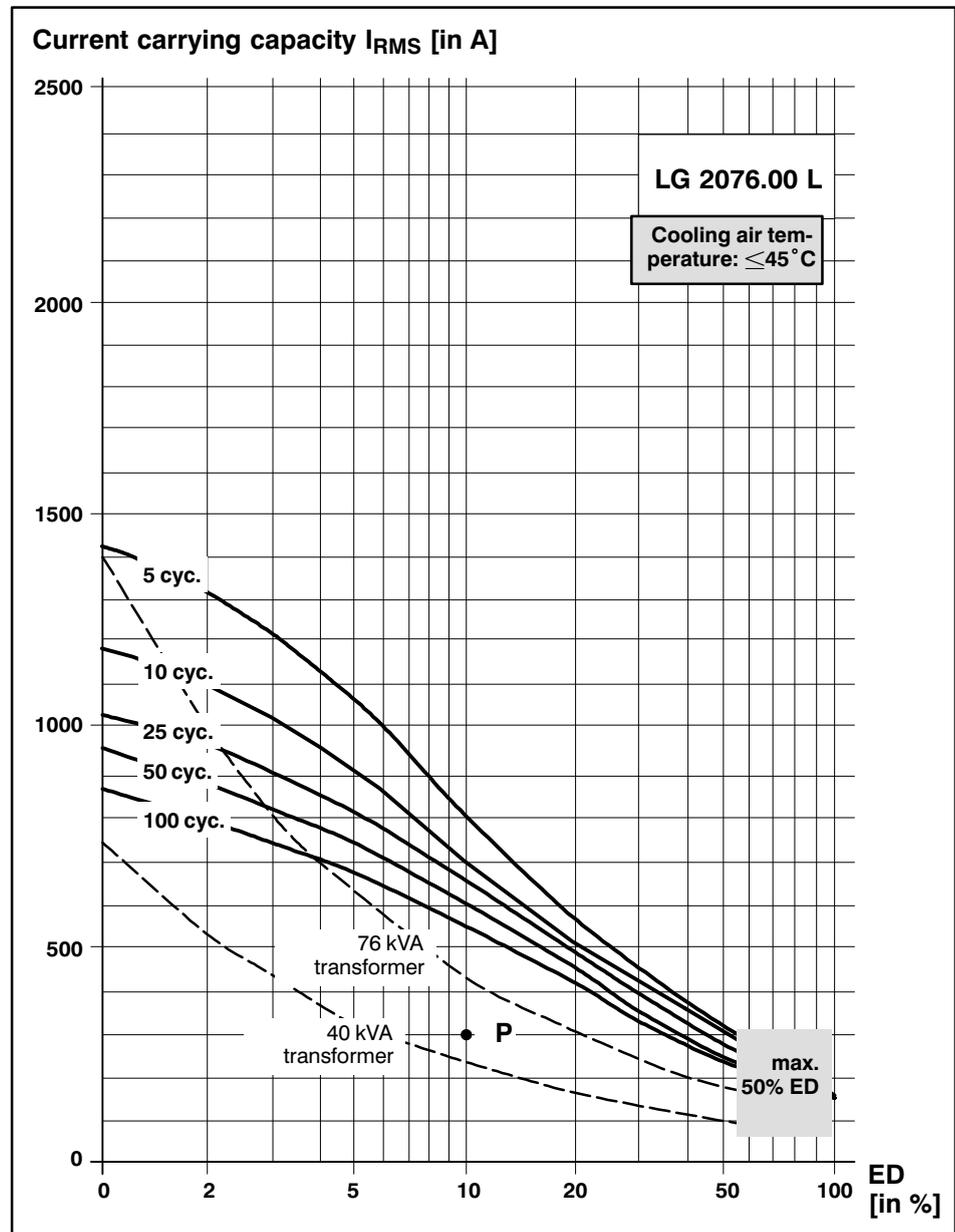
**Example:** Weld data of the machine: 76 kVA
