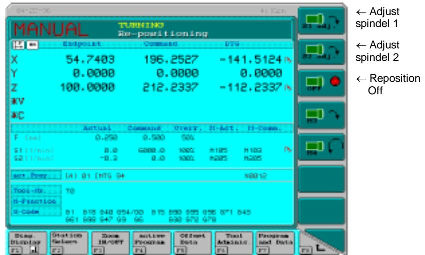
Figure 2-2: Example: REPOS screen for repositioning and NC-block restart.
