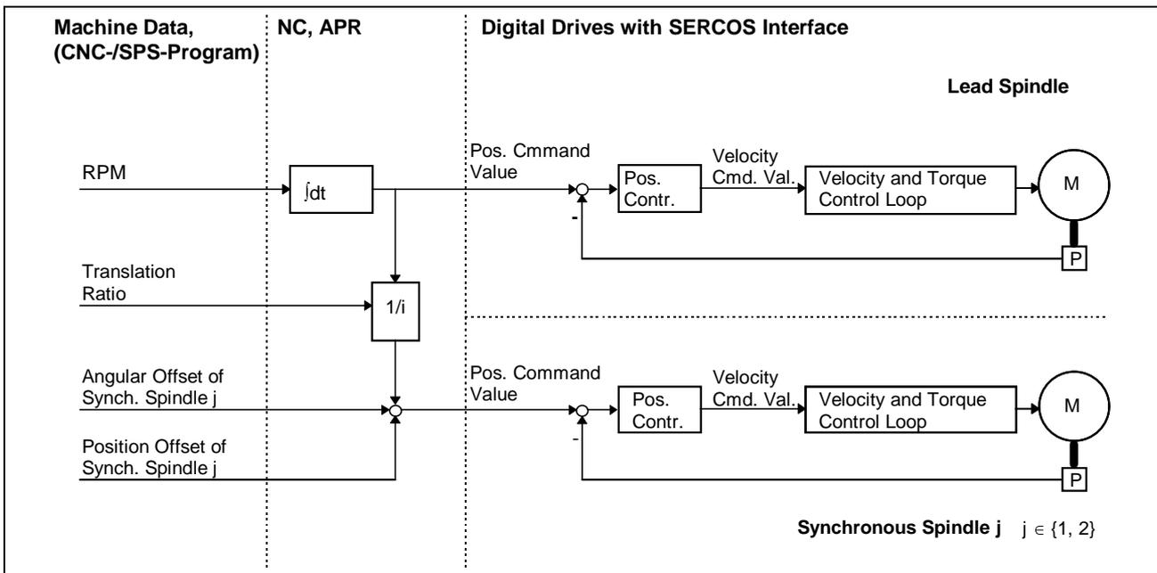
Fig. 3-1: Operation of the angular difference and synchronous position offset.
