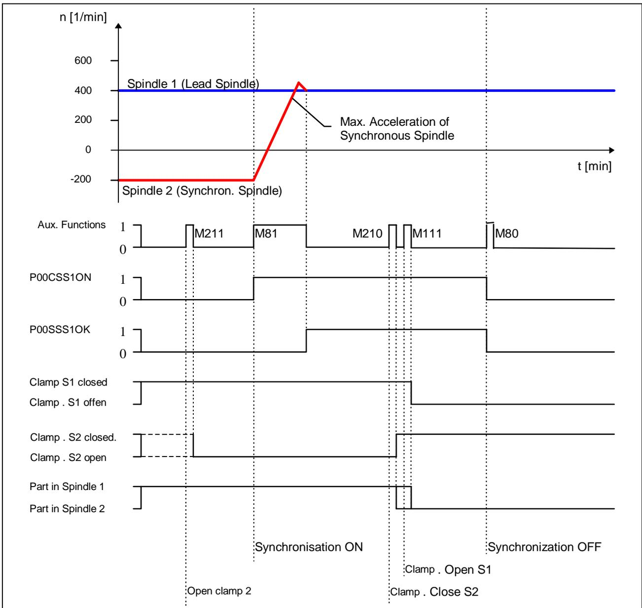
Fig. 6-1: Transferring a part from spindle 1 to spindle 2.
