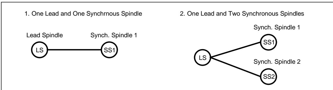
Fig. 3-2: Legal spindle configurations within a process.
