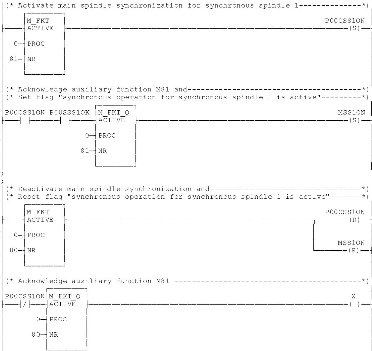
The clamping fixture for spindle 2 (synchronous spindle 1) is closed and opened via the M-functions 'M210' and 'M211'. It is important that during synchronous operation the clamping fixture only be closed when spindle 2 (synchronous spindle 1) is completely in synch with spindle 2 (lead spindle 1) (P00SSS1OK).
