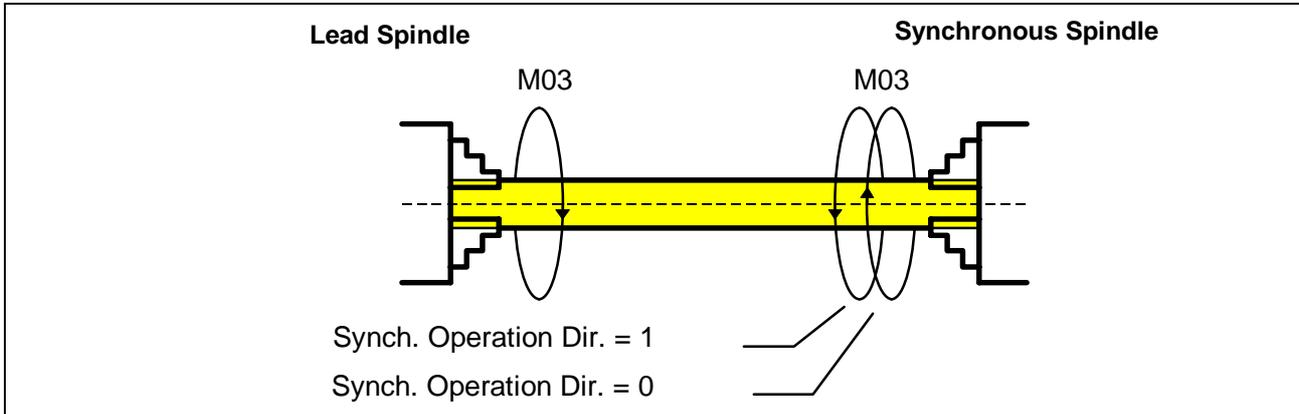
Fig. 4-1: Synchronized operation direction of rotation.
