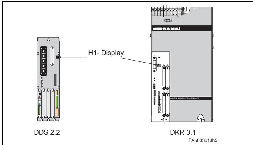
Fig. 1-2: H1-Display on DDS and DKR drives
