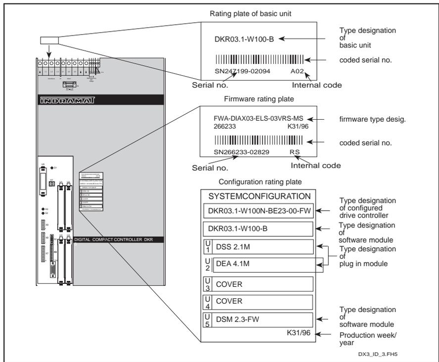
Fig. 4-3: Rating plate of the DKR03.1 (Example)
