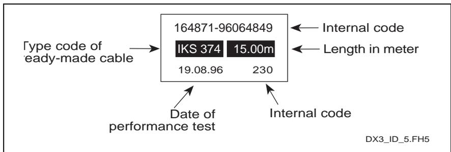
Abb. 4-5: Rating plate of ready-made INDRAMAT cables (Example)
