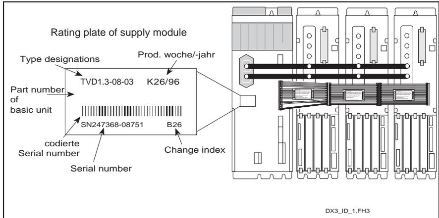
Fig. 4-1: Rating plate on the supply module (Example)
