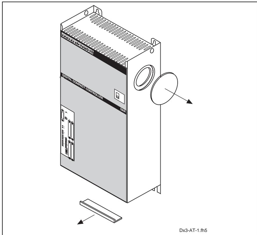
Abb. 4-6: Converting the DKR04 to control cabinet cooling!
