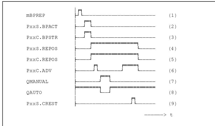
Figure 6-8: Interaction of the relevant signals for NC program restart and subsequent multi-block retrace
