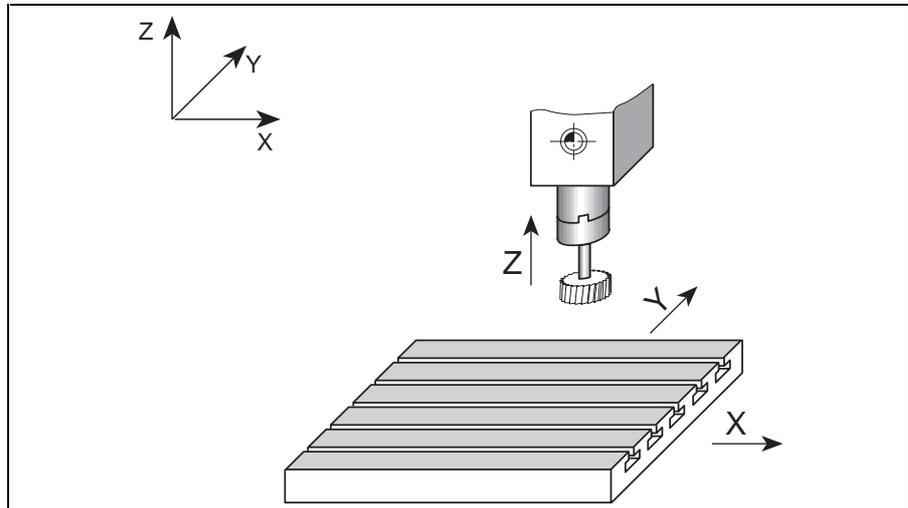
Figure 7-9: Structure of the milling machine
