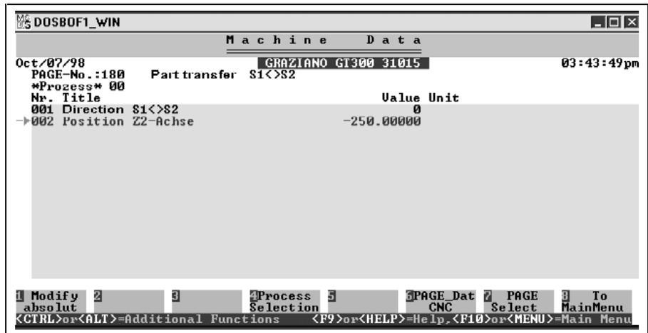
Figure 7-17: Machine data page for parts transfer
