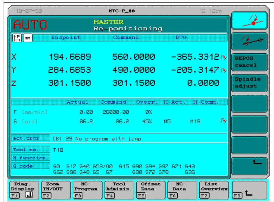
Figure 2-4: 'Re-positioning' screen
