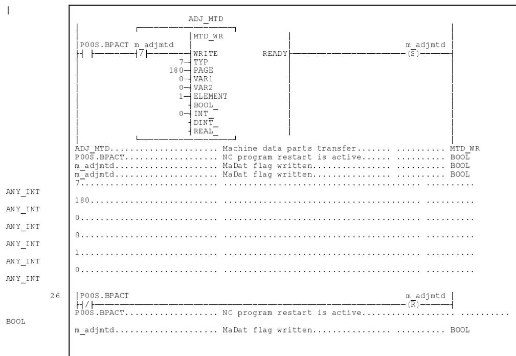
Figure 7-18: SPS function block for parts transfer
