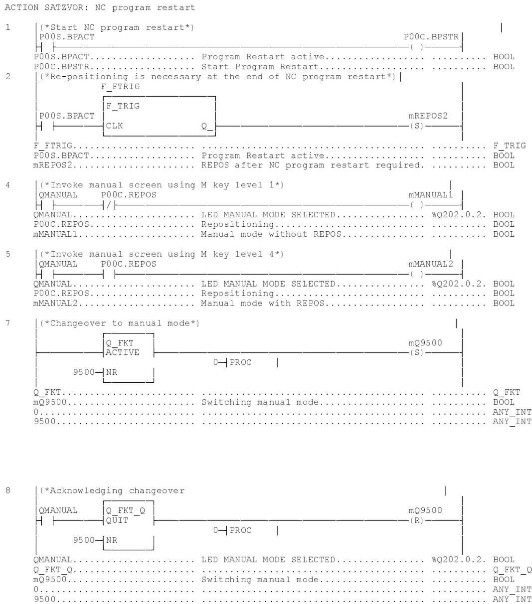
Figure 7-13: SPS program segment for NC program restart
