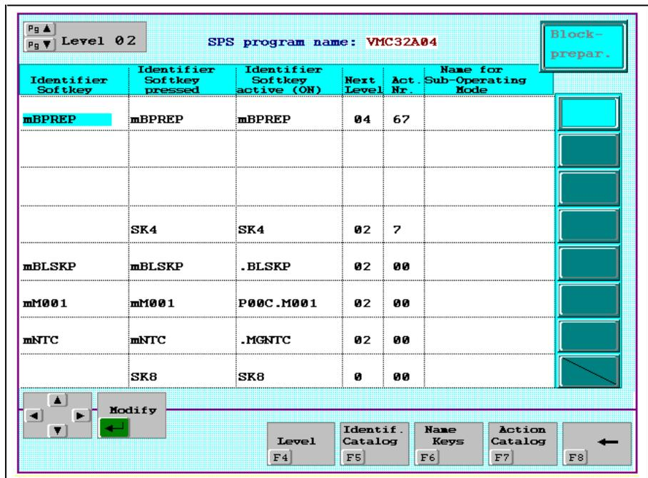
Figure 7-11: Entering the M key 'NC program restart'
