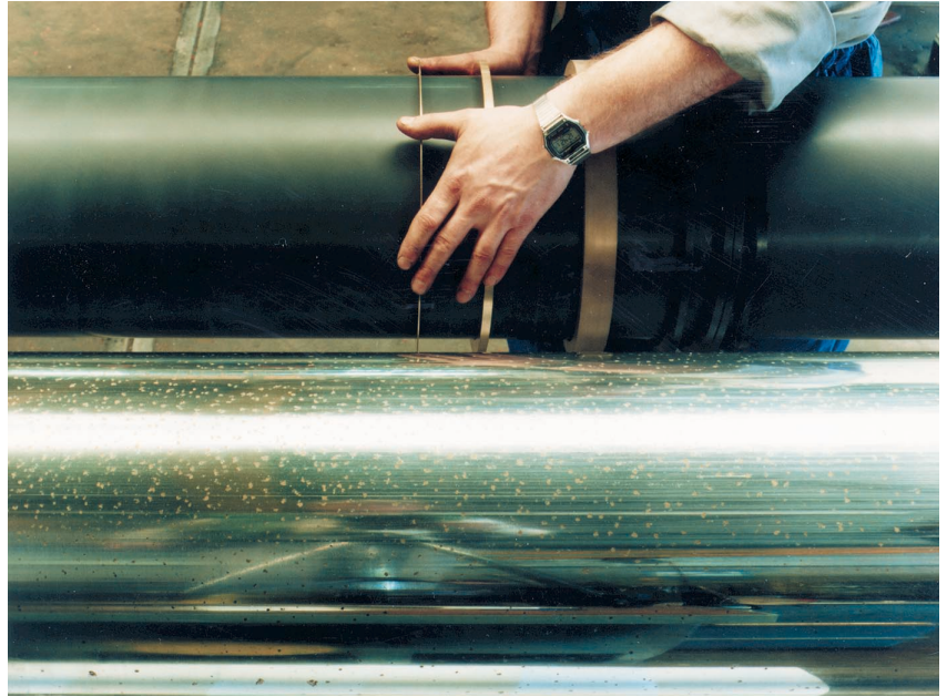
Typical corrosion on chromium plated piston rods
