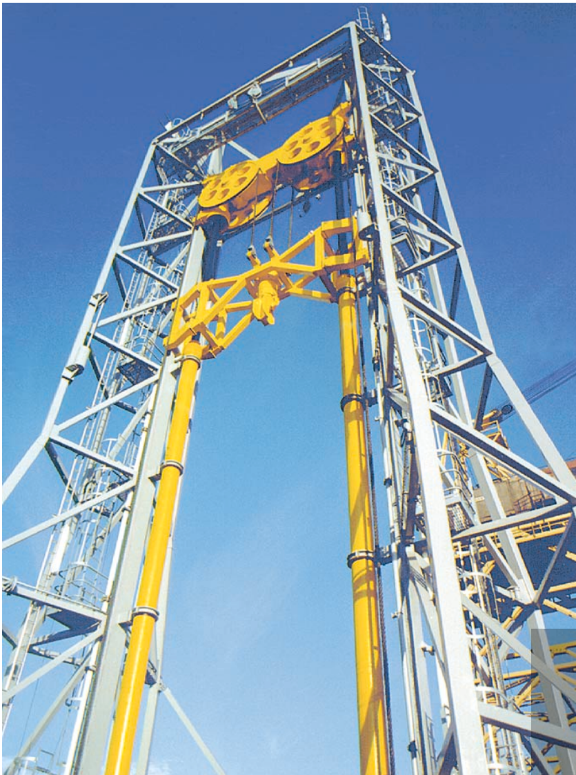
Ram Rig cylinders on a Semi-submersible Rig
