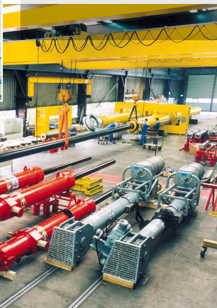
Ceramax cylinders for the Storm Surge Barrier in the Hartel canal at Rotterdam
