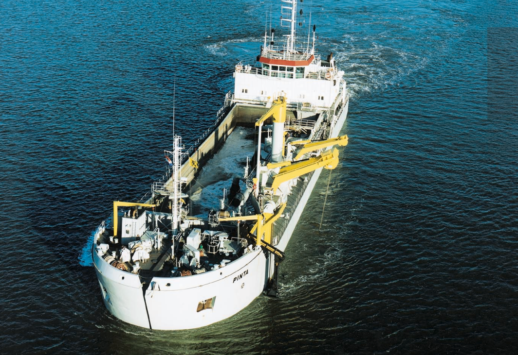
Split hopper dredger with ABS Hydro Cylinders
